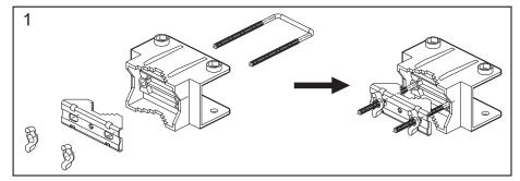
First insert the U-bolt into the fixed mount. Then mount the fixed U-shaped mount, tighten with the hex nuts as shown in the diagram above.
