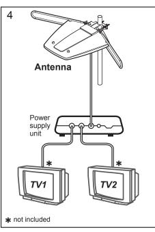
Connect your antenna to the power supply unit, and the power supply unit to one or two TVs.
