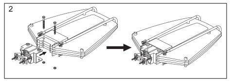
Insert the assembled fixed mount screw into the antenna body screw notch, tighten with the nuts underneath the fixed mount as shown in the diagram above.
