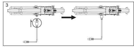
Tighten the cable onto the F-connector. After it is tightened, insert the water seal onto the antenna body as shown in the diagram above.
