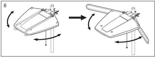
Unscrew the wing screw and deploy the two antennas, adjust the antennas for an optimal reception.
