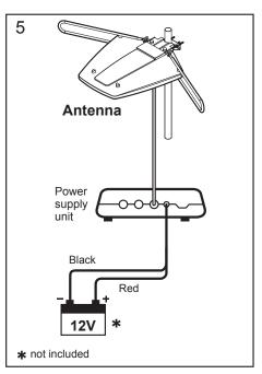
Plug the power supply unit into a wall outlet or use the red and black cable for the power supply by a car battery\*.
